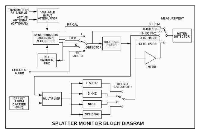
A 3-1/2 digit thumbwheel switch labeled CARRIER kHz adjusts the operating frequency of the Splatter Monitor from 450 kHz to 1800 kHz. Simple jumper changes allow operation at either 9 kHz or 10 kHz channel spacing. When tuned to 450 kHz, the Splatter monitor can be connected to the 450 kHz IF output of a synthesized receiver, taking advantage of the Splatter Monitor's synchronous detectors to evaluate the I and Q modulation of received stations.
